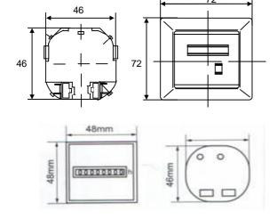
48x48mm no front plate 72x72mm with front plate
